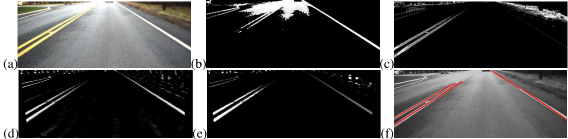
Figure 6: Stages of Lane Detection (a-f).
