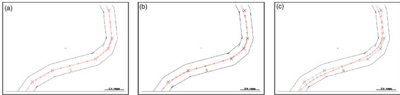
Figure 20. Smoothing of the RDDF: (a) Adding additional points; (b) the trajectory after smoothing (shown in red); (c) a smoothed trajectory with a more aggressive smoothing parameter. The smoothing process takes only 20 seconds for the entire 2005 course.
