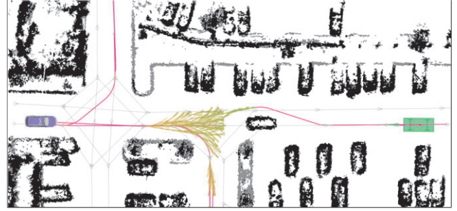
Fig. 11. Best viewed in color. Combining the topological graph search and the free-space path planning. The Reed–Shepp transitions to and between nodes of the lane-network graph \mathcal{G} are shown in purple. The forward free-space expansions are shown in yellow.
